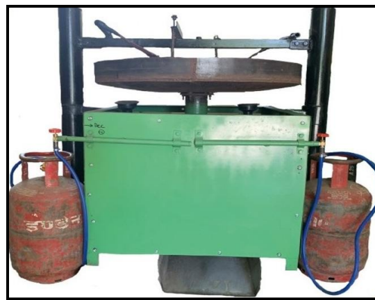
Fig. 1. Images of the popped makhana grading machine (Fig. 1a) and primary roasting machine (Fig. 1b).
