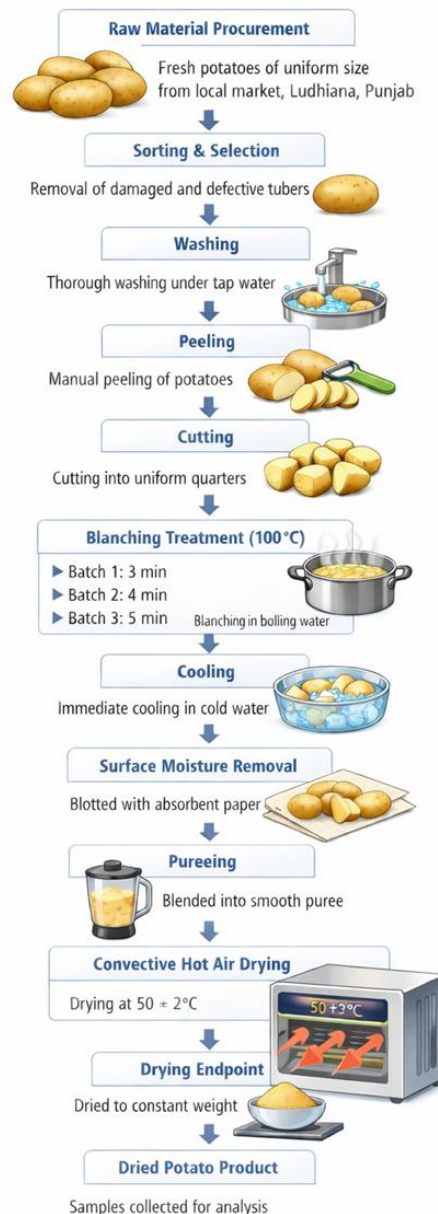
Figure 1. Process flow diagram for convective hot air drying of blanched potato
