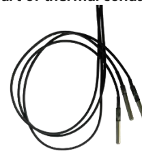
(c) DS18B20 Temperature sensors
